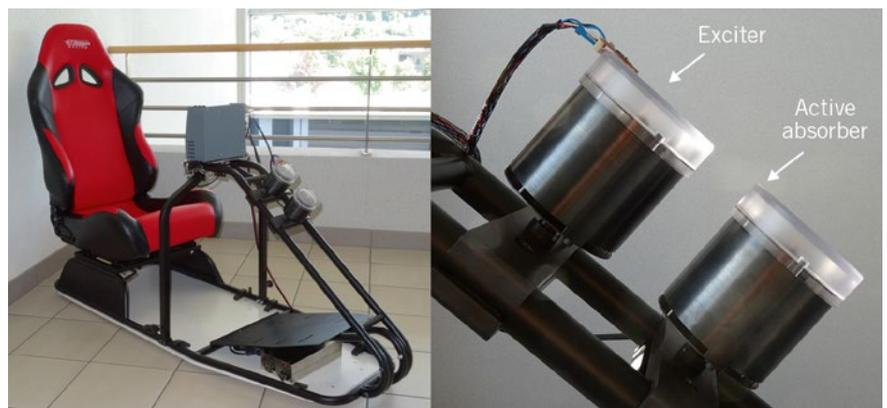
**FIGURE 5** Interactive demonstrator (left) featuring moving magnet exciter and active absorber (right) (© MMT)
